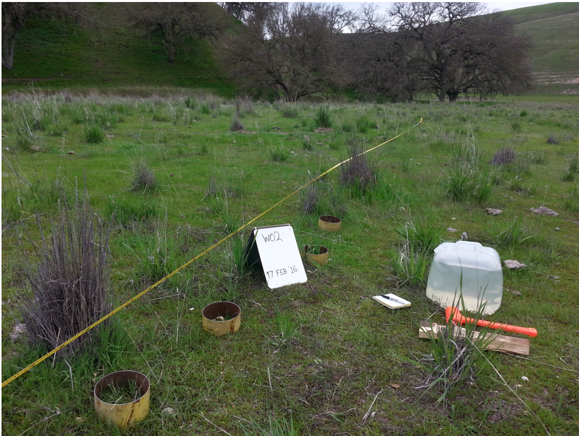
Infiltration rings along a transect.
